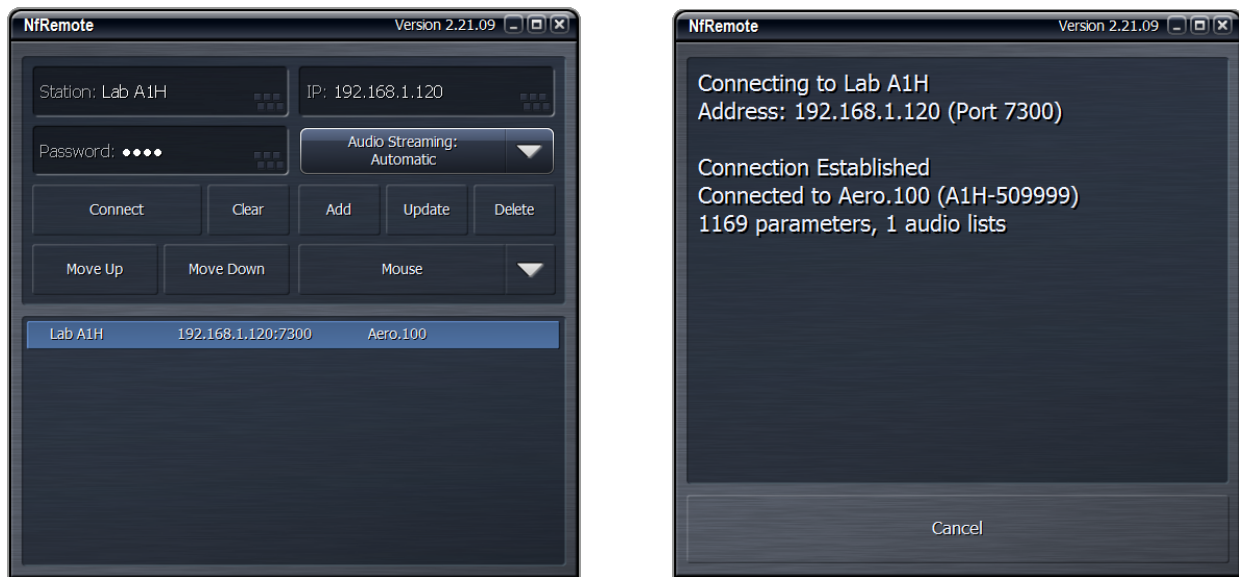
Figure 2-2 Left: Remote control setup screen; Right: AERO.100 negotiates connection with remote
