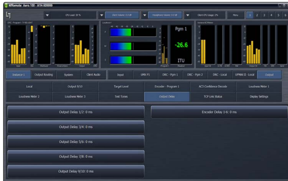
Figure 1-13 Output Delay settings available for each instance
