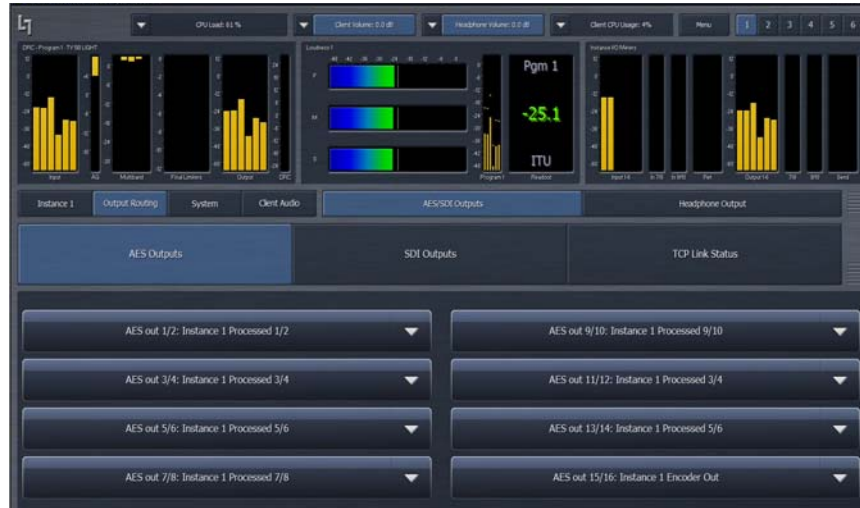
Figure 1-8 The AES and SDI Outputs tabs allow source selection for each physical output
