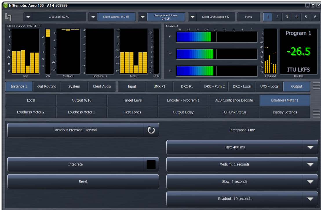
Figure 2-9 Settings for the program-specific ITU meter
