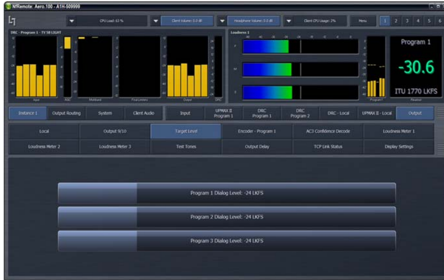
Figure 1-17 Dialog level (dialnorm) is set under the Target Level tab
