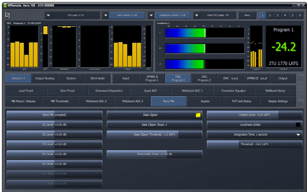
Figure 1-19 Adjusting Output Level so the meter matches the target
